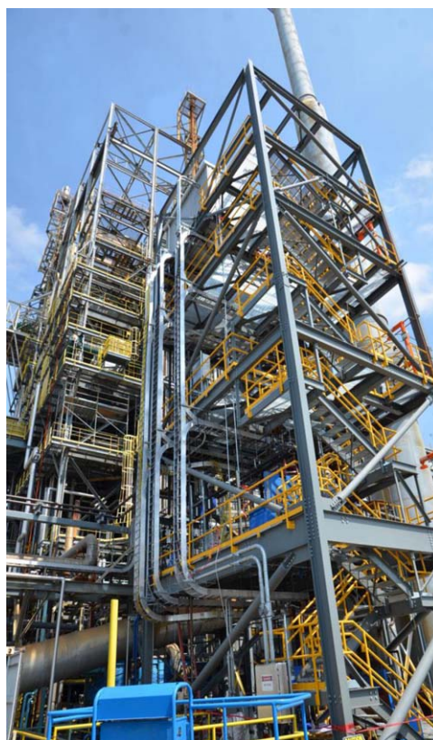
Figure 10. Photo of the OSU high-pressure SCL pilot plant at the NCCC in Alabama for hydrogen generation and CO 2 capture.
